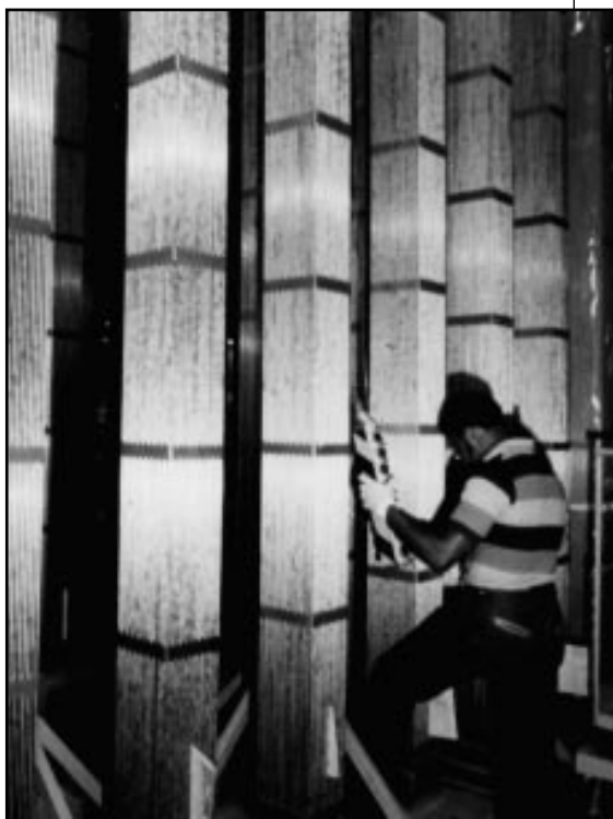
From 64 to 256 fuel pins are arranged together to form a fuel assembly.
