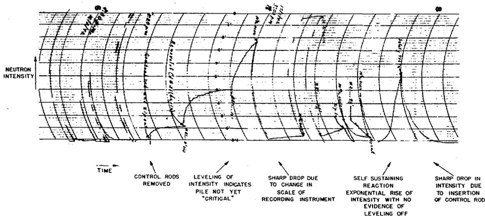
*The "birth certificate" of the Atomic Age. The galvanometer chart that indicated the rise in neutron intensity associated with the first controlled chain reaction.*
