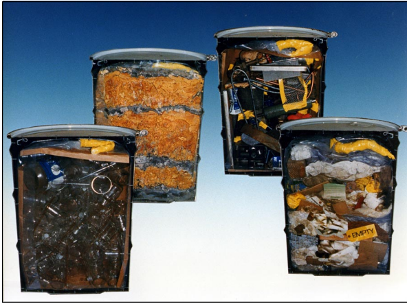
This cutaway view of barrels of LLW shows how clothing, equipment, and solidified sludge are packaged in a dry, solid form.
