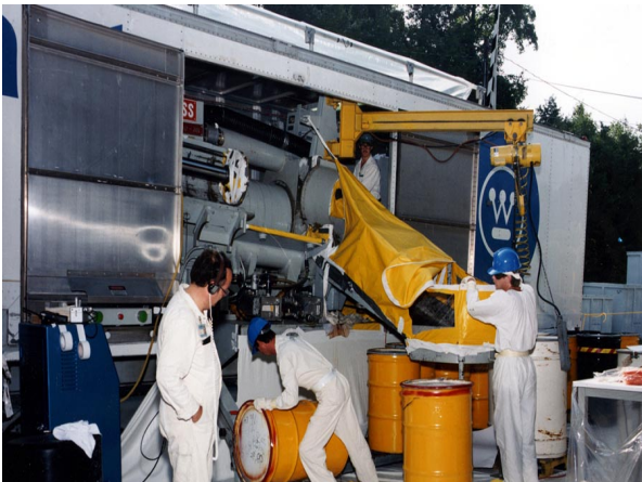
Volume reduction can be achieved with super-compactors, which use hydraulic force to squeeze drums of LLW down to less than one-fourth of their original size.
